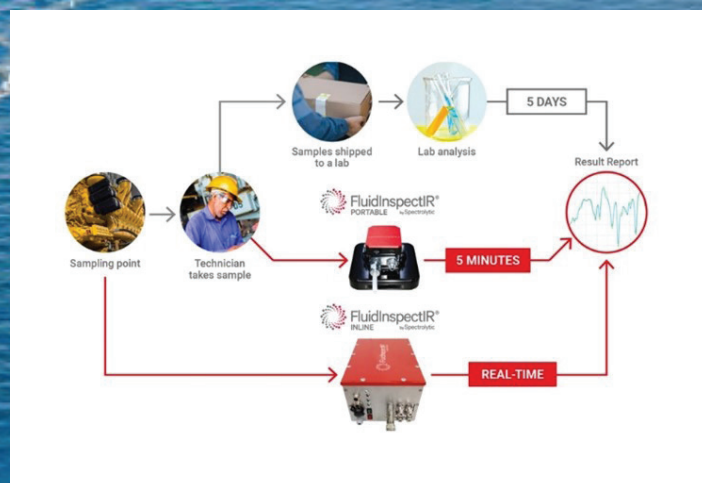
Figure 1: Typical oil analysis process in an industrial environment and the positive effects of at-line or real time oil analysis
